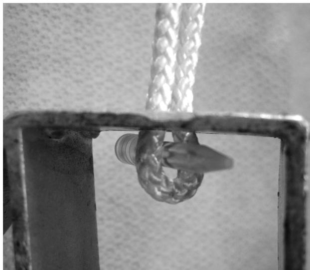
**Figure 1** Experimental set-up using a looped polypropylene rope to tension the Bio-Transfix pin.
