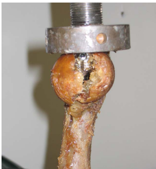
Figure 3 Head splitting fracture observed in ITST specimen during axial loading to failure.
