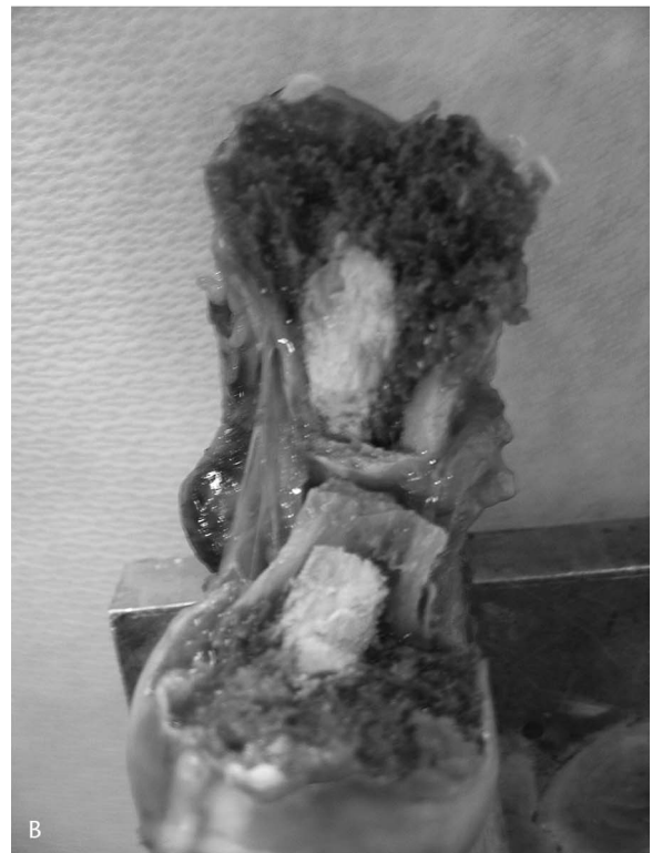
FIGURE 5. Failure with vertical loading occurred most commonly by fracture through the center of the femoral neck.
