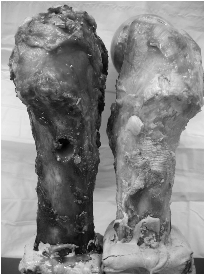
FIGURE 2. Femoral neck defect augmented with Norian calcium phosphate cement (right) and its untreated control (left).
