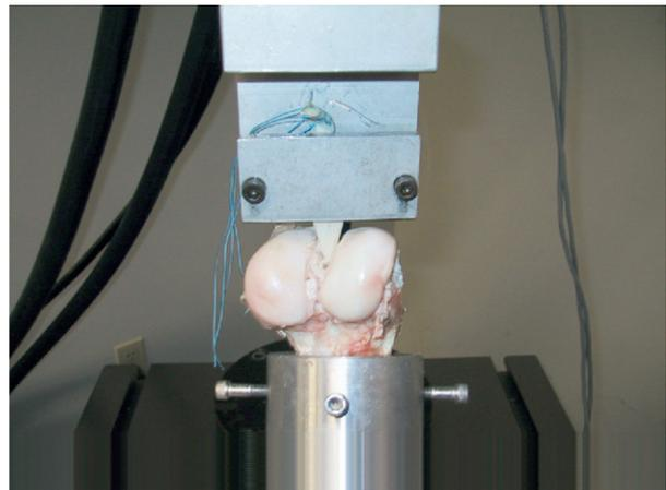
**FIGURE 3.** Testing apparatus with mounting of distal femur (model 8521; Instron).
