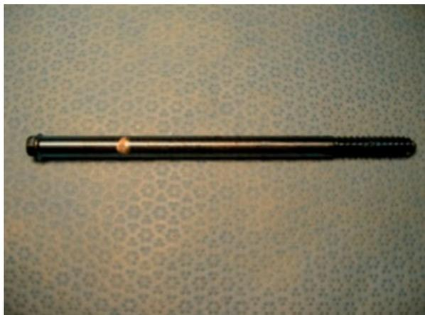
**Figure 5.** Indentation of the superior lag screw observed in the region of the medial screw hole during loading.
