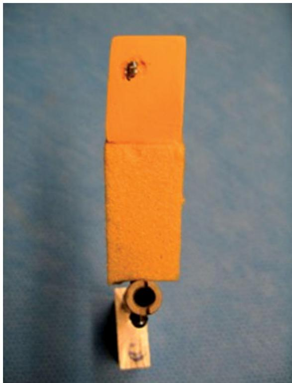
**Figure 4.** Penetration of the superior aspect of the specimen head component by the superior lag screw after 10,000 cycles of vertical loading. Superior lag screw penetration was observed in all three specimens whose head components had a compressive strength of 0.91 MPa heads and in one specimen with a 2.2 MPa head.
