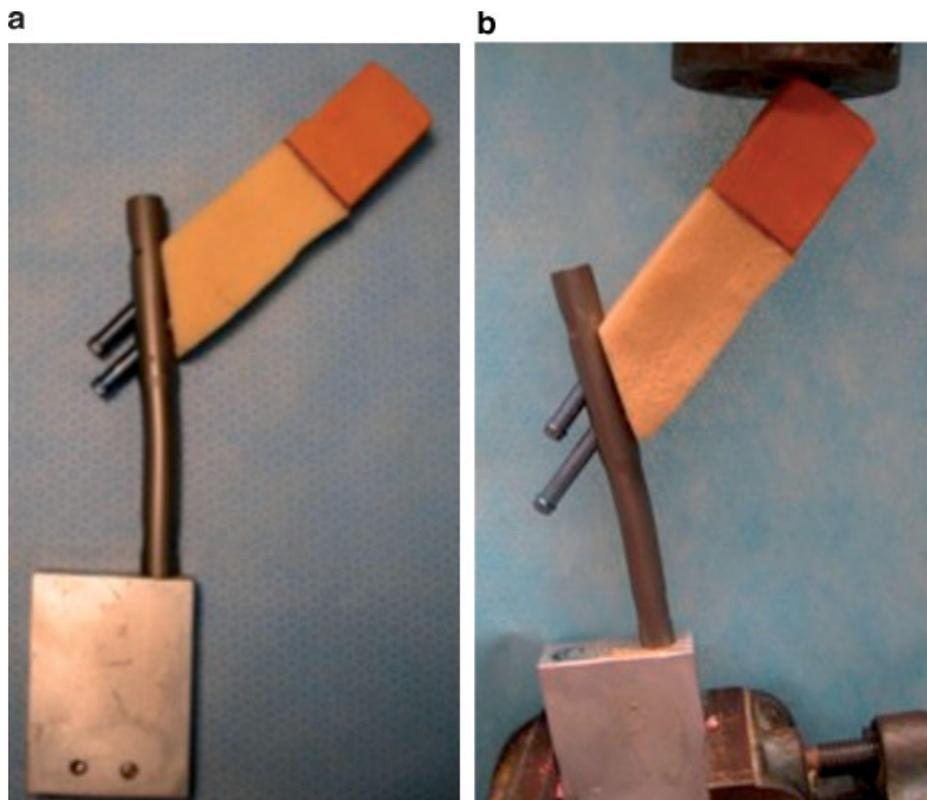
**Figure 2.** (a) TAN-Sawbones construct (neck component of 0.91 MPa compressive strength and head component of 8.8 MPa compressive strength). (b) Application of a vertical load resulted in varus angulation of the implant-neck/head interface. Cyclic loading led to 11 mm of lateral migration of the inferior lag screw after 10,000 cycles.
